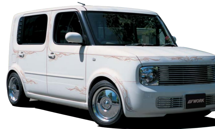
[SIZE] FRONT:15inchX6.5J OFFSET +48mm (A) TIRE:185/55-15 REAR:15inchX6.5J OFFSET +40mm (A) TIRE:185/55-15 COLOR:クロームメッキ (M) ※ファンダー加工
